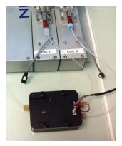
Our microfluidic system allows fast and simple rheological measurements, using minute amounts of sample. The microchannel configuration allows viscosity analysis under high shear rates and under strong confinement, mimicking your real process conditions.
